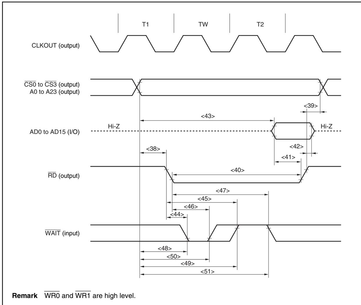
**(b) Write cycle (CLKOUT asynchronous): In separate bus mode**
