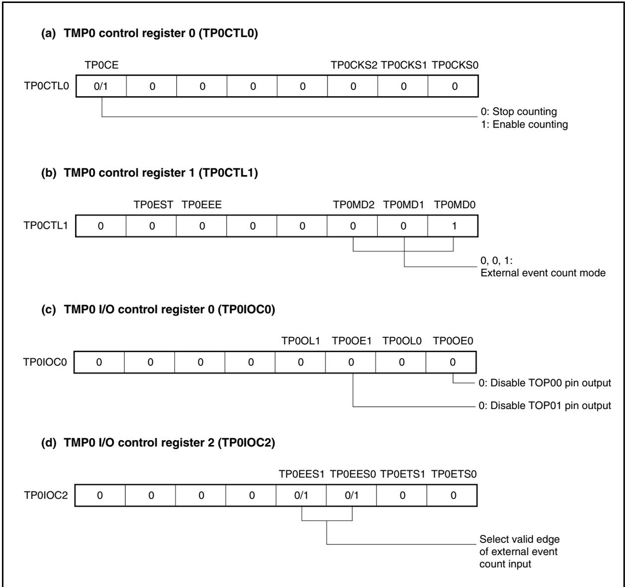
**Figure 7-11. Register Setting for Operation in External Event Count Mode (2/2)****(e) TMP0 counter read buffer register (TPOCNT)**
