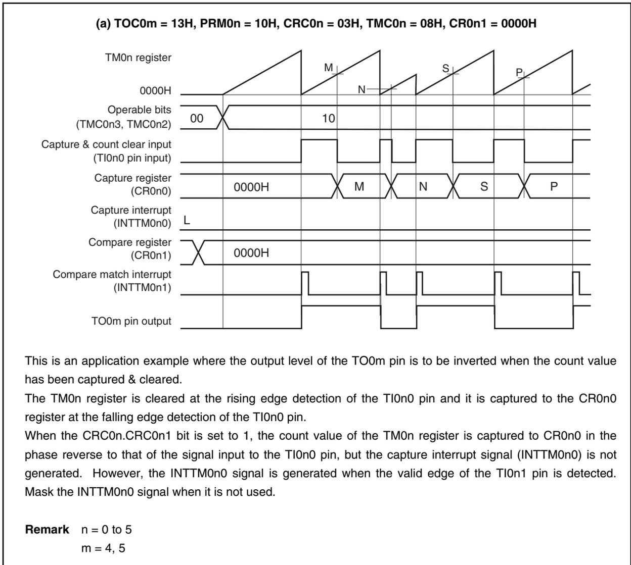
**Figure 8-18. Timing Example of Clear & Start Mode Entered by TIO<sub>n</sub>0 Pin Valid Edge Input
