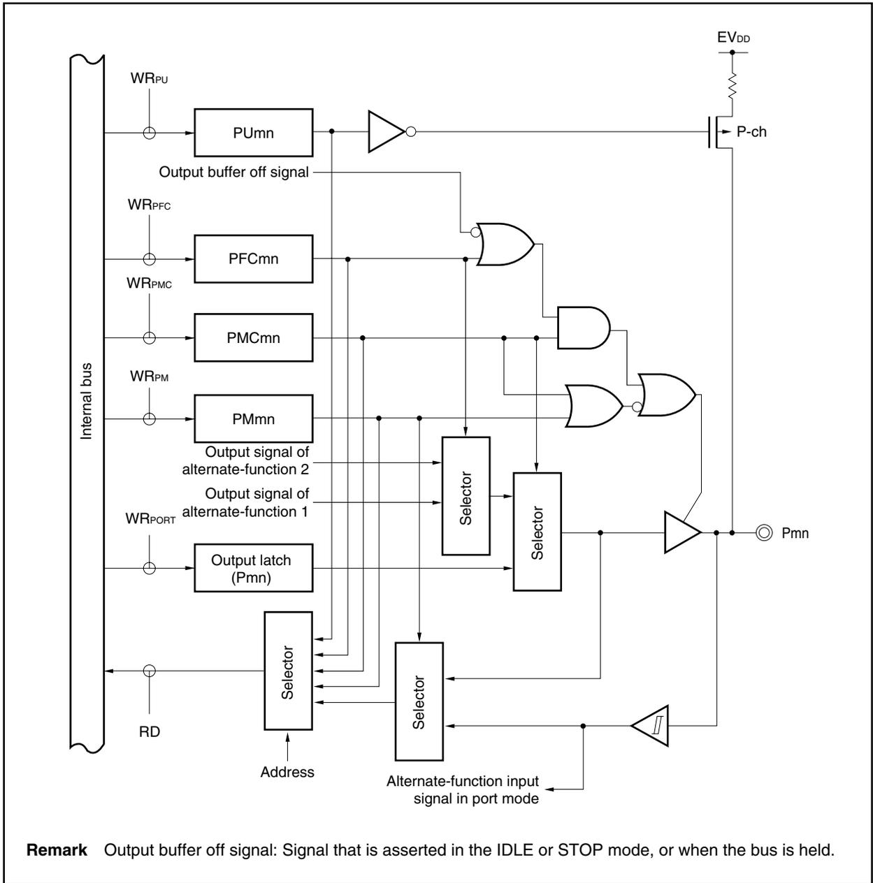
Figure 4-15. Block Diagram of Type E-4
