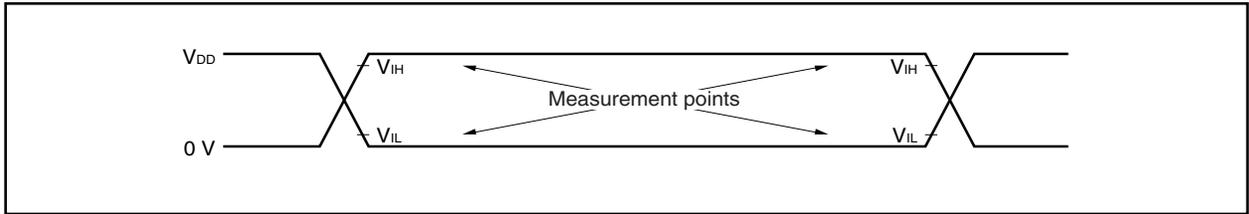
**AC Test Output Measurement Points**
