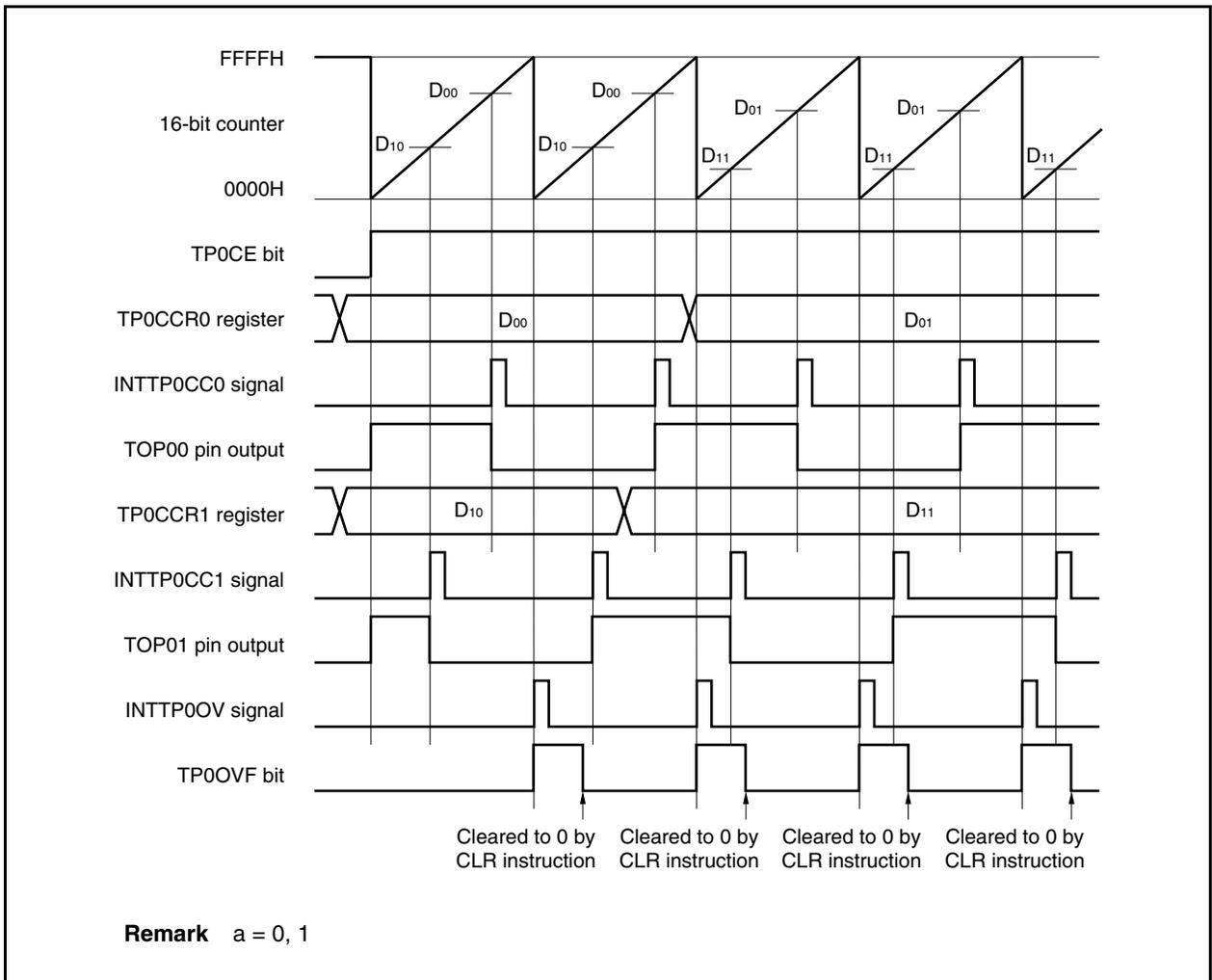
When the TP0CE bit is set to 1, the 16-bit counter starts counting. When the valid edge input to the TIP0a pin is detected, the count value of the 16-bit counter is stored in the TP0CCR<sub>a</sub> register, and a capture interrupt request signal (INTTP0CC<sub>a</sub>) is generated.
