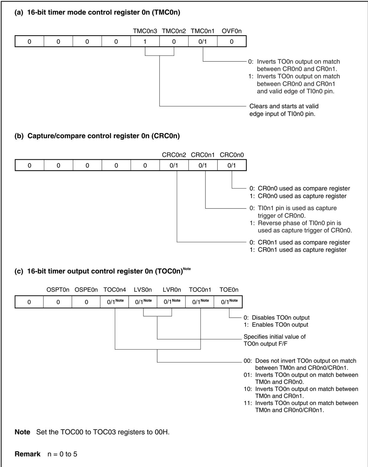
Figure 8-21. Example of Register Settings in Clear & Start Mode Entered by TIO<sub>n</sub> Pin Valid Edge Input (2/2)**(d) Prescaler mode register 0n (PRM0n)**
