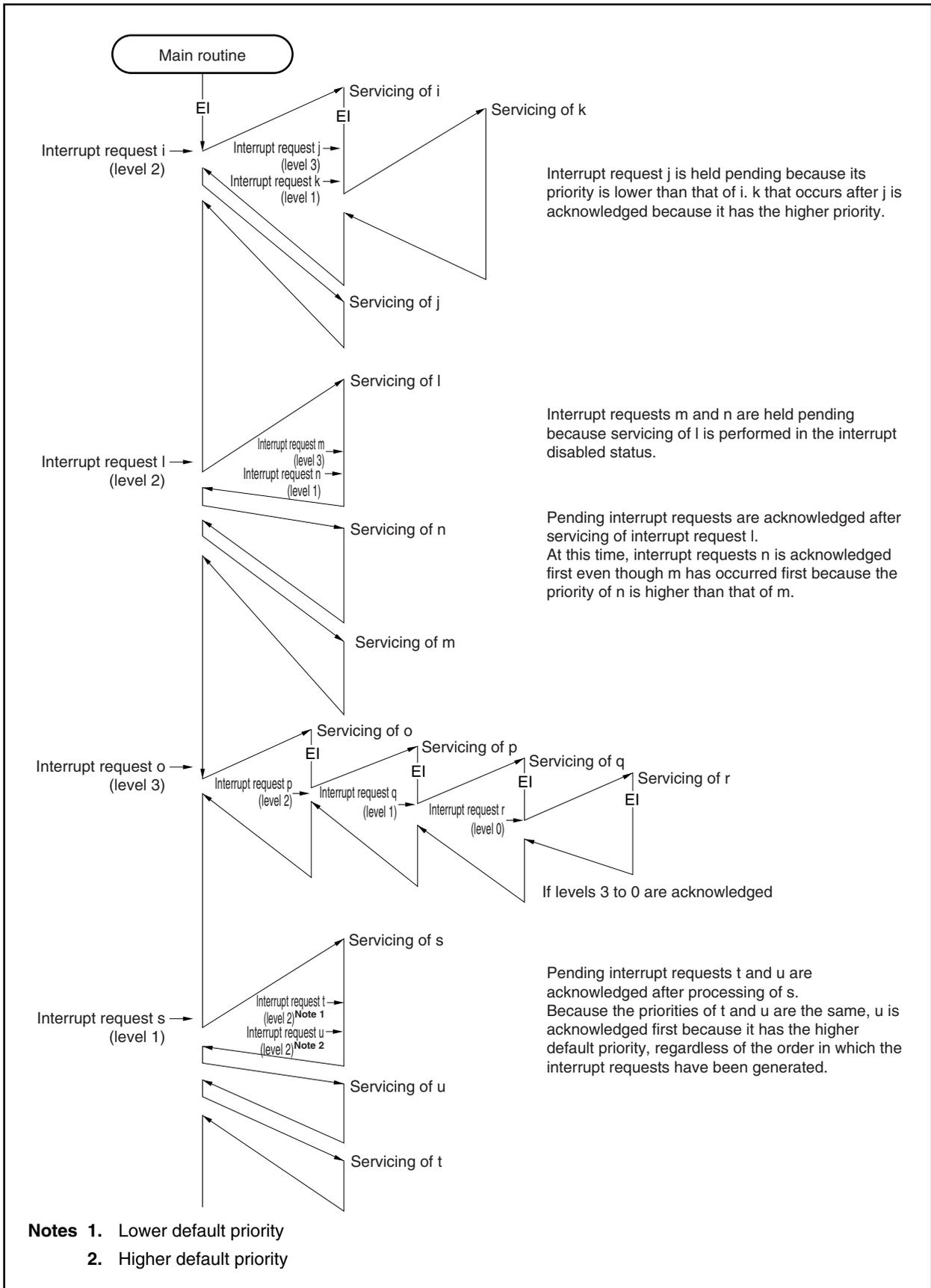
Figure 20-7. Example of Servicing Simultaneously Generated Interrupt Request Signals
