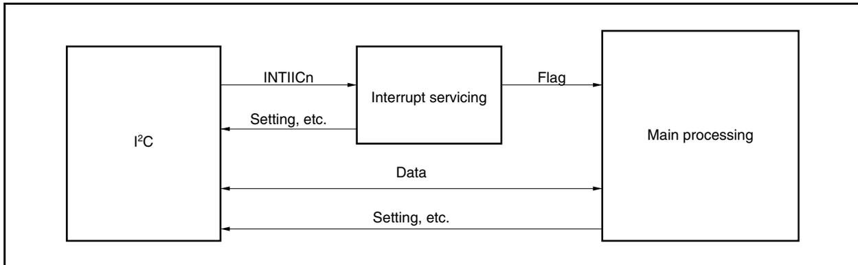
Therefore, the following three flags are prepared so that the data transfer processing can be performed by transmitting these flags to the main processing instead of the INTIICn signal.
