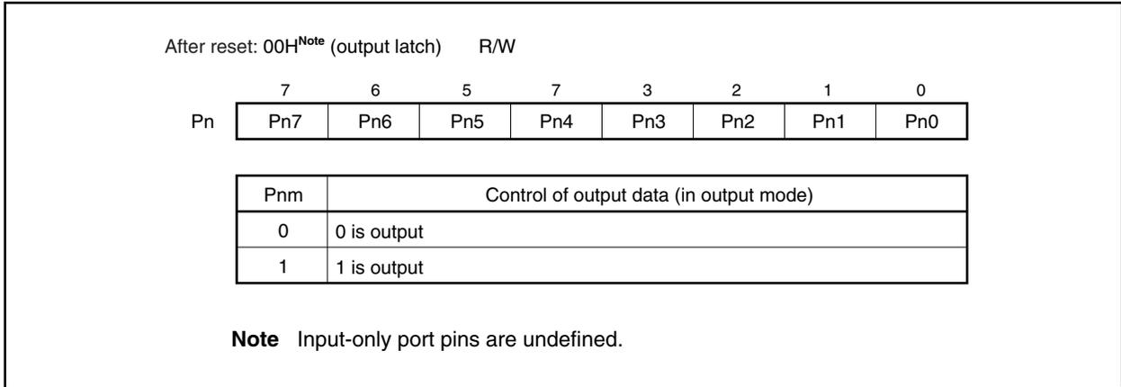
Writing to and reading from the Pn register is executed as follows depending on the setting of each register.
