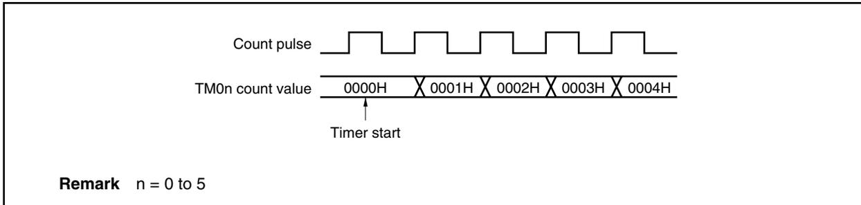
**(3) Setting CR0n0 and CR0n1 registers (in the mode in which clear & start occurs upon match between TM0n register and CR0n0 register)**
