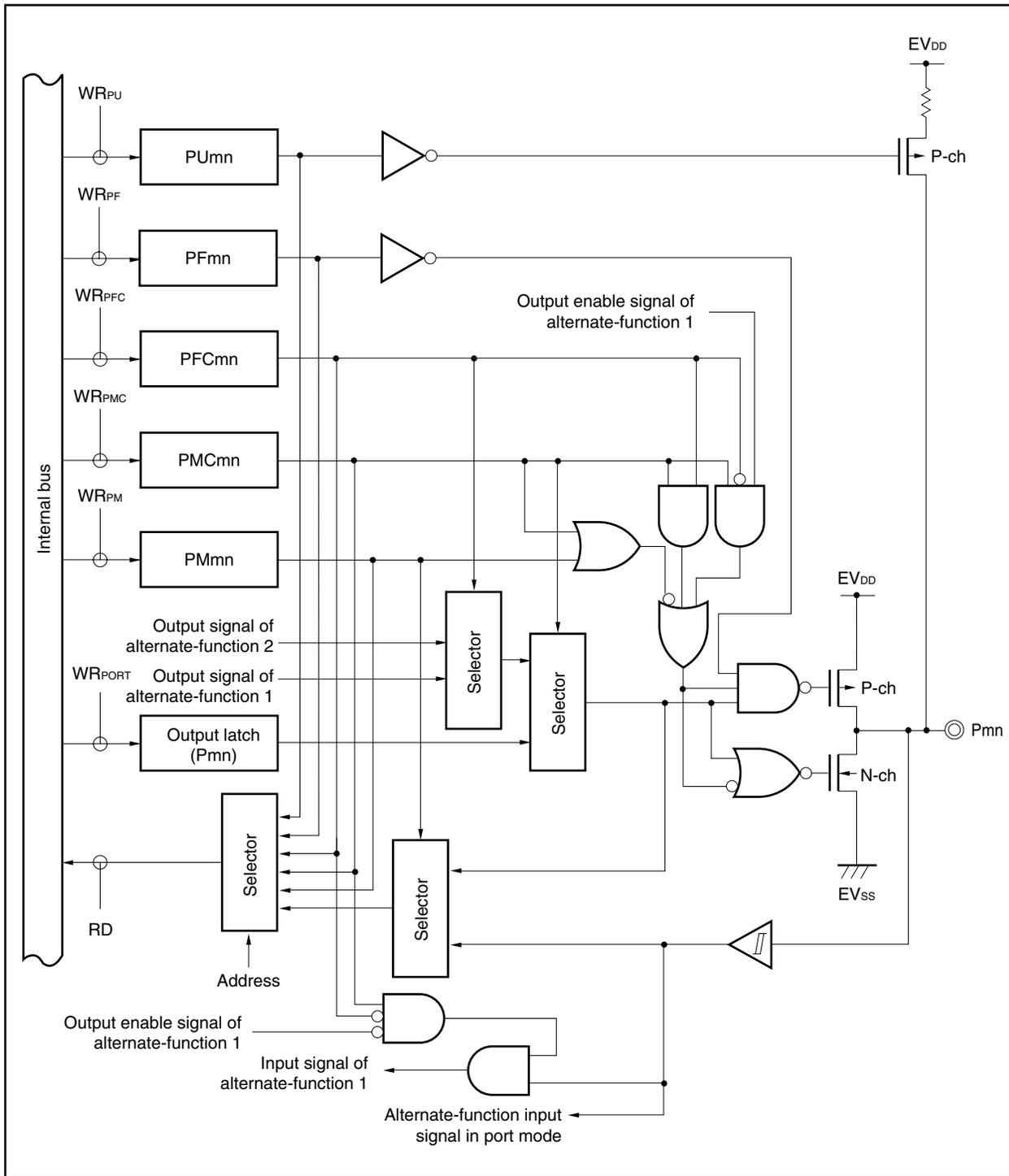
Figure 4-22. Block Diagram of Type G-3
