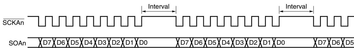
**Cautions** 1. Because, in the repeat transmission mode, a read is performed on the buffer RAM after the transmission of one byte, the interval is included in the period up to the next transmission. As the buffer RAM read is performed at the same time as CPU processing, the interval is dependent upon the ADTIn register.
