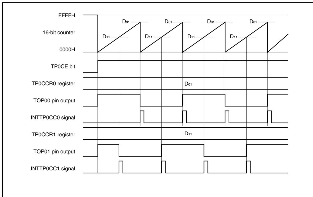
If the set value of the TP0CCR1 register is greater than the set value of the TP0CCR0 register, the count value of the 16-bit counter does not match the value of the TP0CCR1 register. Consequently, the INTTP0CC1 signal is not generated, nor is the output of the TOP01 pin changed.
