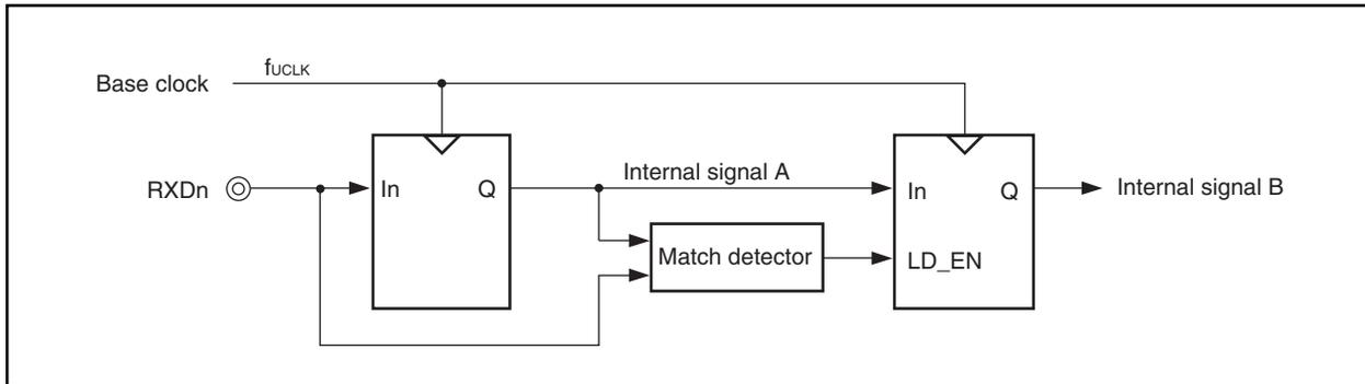
**Figure 16-12. Timing of RXDn Signal Judged as Noise**
