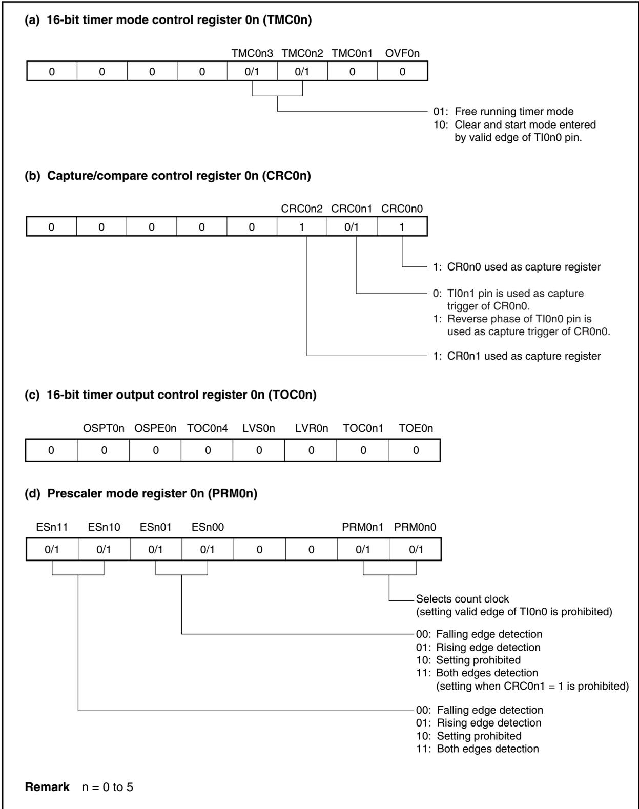
Figure 8-42. Example of Register Settings for Pulse Width Measurement (2/2)
