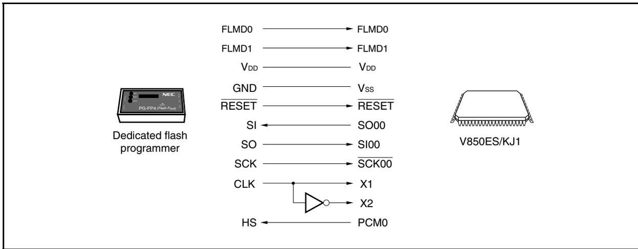
The dedicated flash programmer outputs the transfer clock, and the V850ES/KJ1 operates as a slave.
