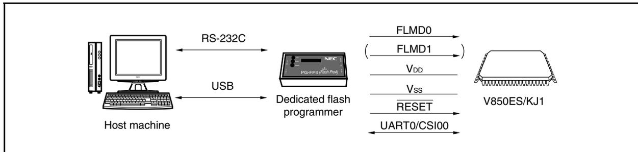
A host machine is required for controlling the dedicated flash programmer.
