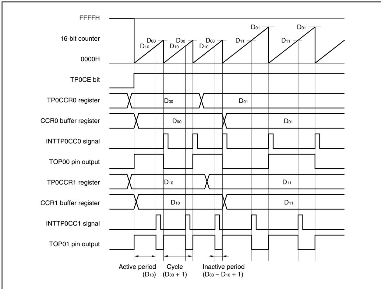
When the TP0CE bit is set to 1, the 16-bit counter is cleared from FFFFH to 0000H, starts counting, and outputs a PWM waveform from the TOP01 pin.
