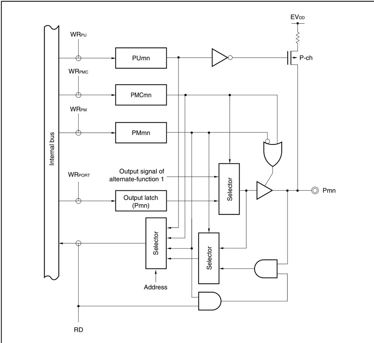
Figure 4-12. Block Diagram of Type E-1
