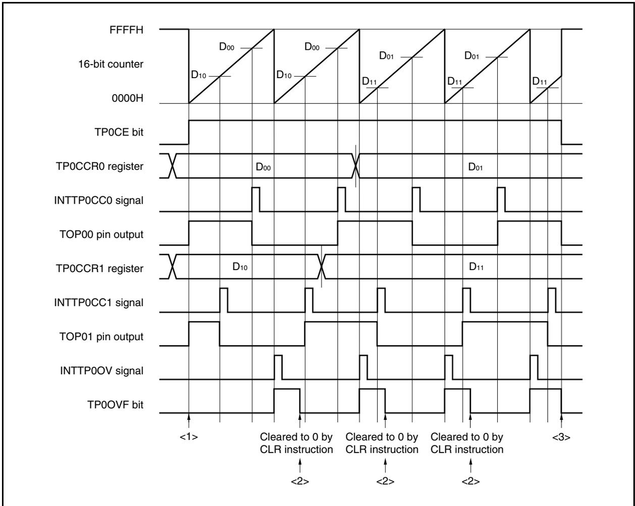
Figure 7-32. Software Processing Flow in Free-Running Timer Mode (Compare Function) (2/2)
