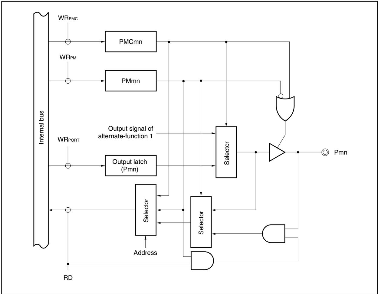
Figure 4-8. Block Diagram of Type C-4
