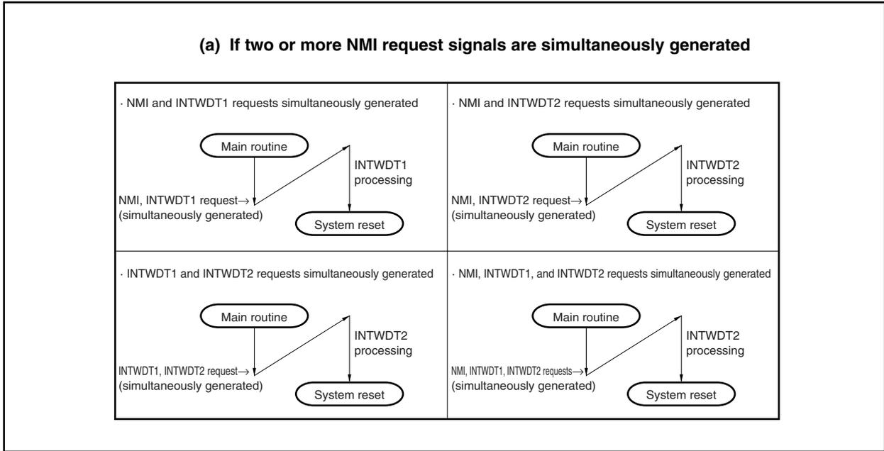
Figure 20-1. Acknowledging Non-Maskable Interrupt Request Signals (2/2)
