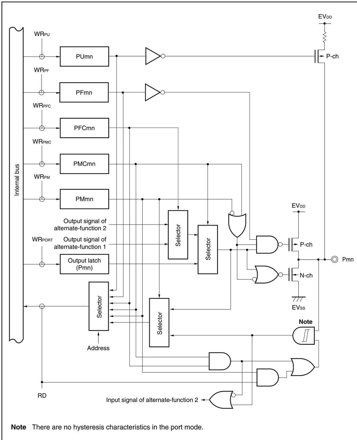
Figure 4-26. Block Diagram of Type G-7-1
