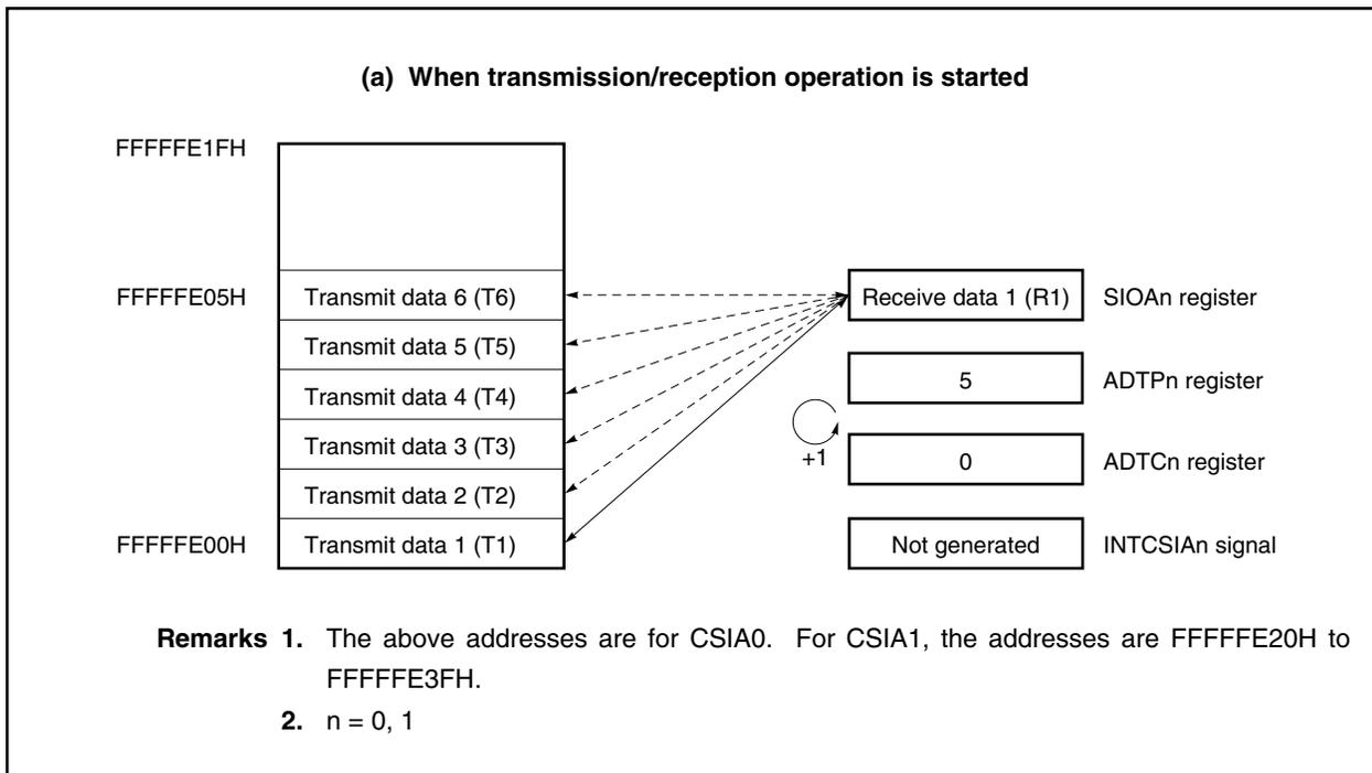
**Figure 18-7. Buffer RAM Operation in 6-Byte Transmission/Reception
