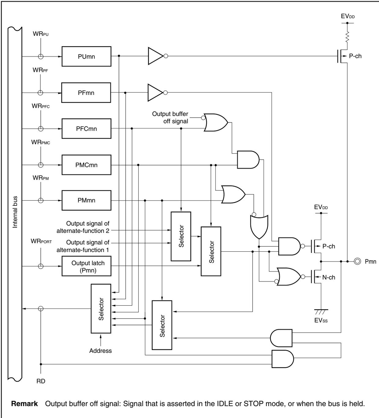
Figure 4-24. Block Diagram of Type G-5
