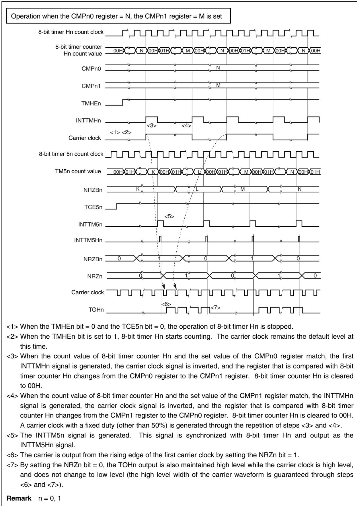
Figure 10-8. Carrier Generator Mode (3/3)
