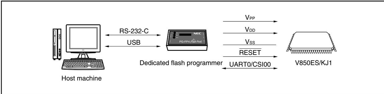
A host machine that controls the dedicated flash programmer is necessary.
