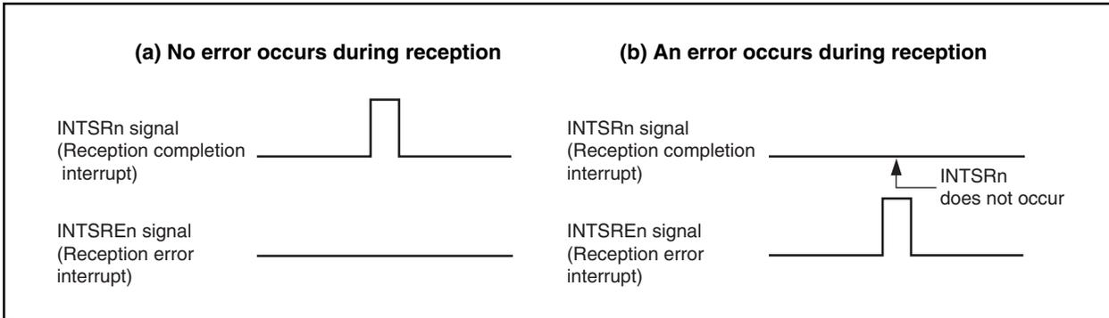
**Figure 16-10. When Reception Error Interrupt Request Signal Is Included in INTSRn Signal (ISRMn Bit = 1)**
