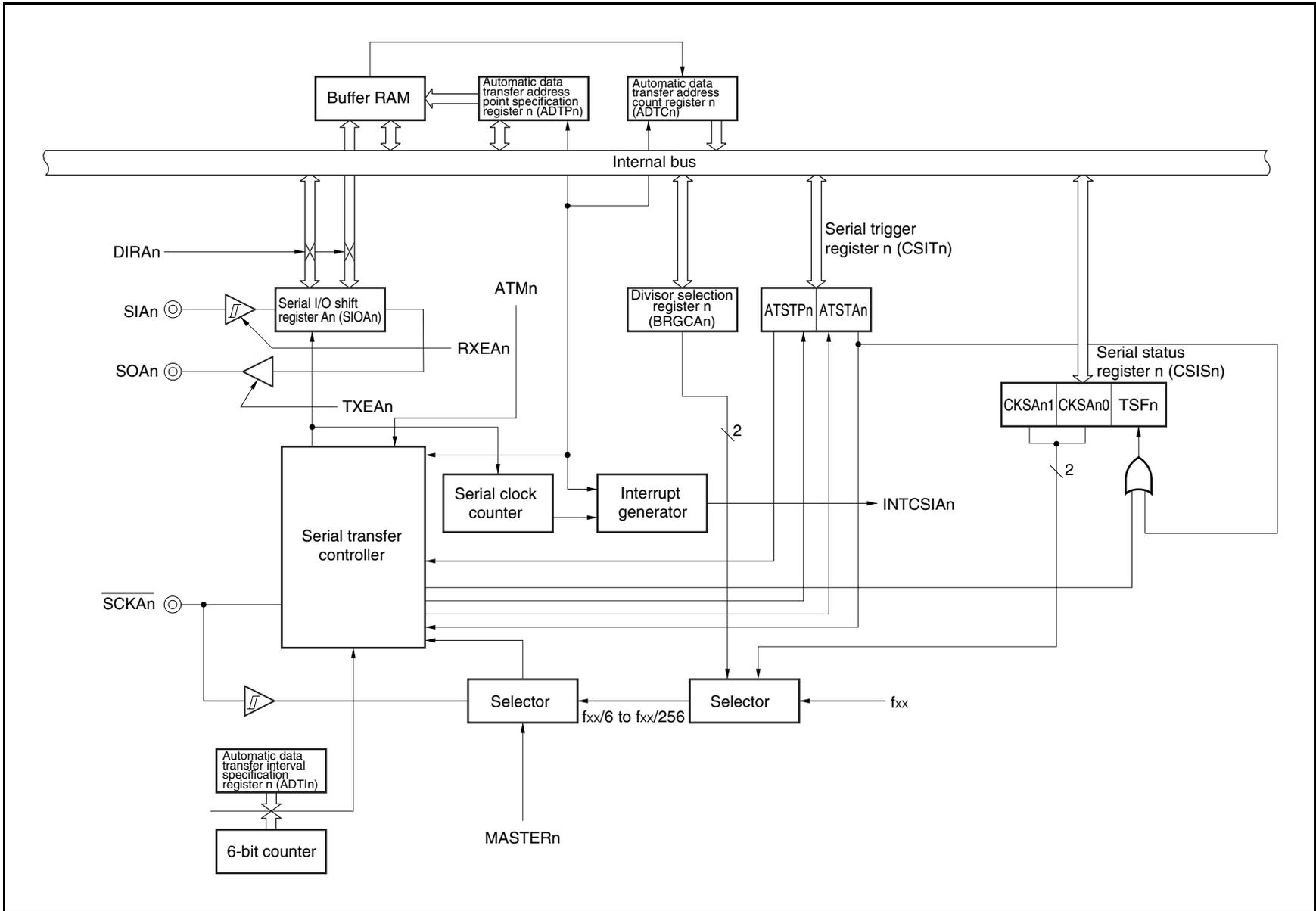
**(1) Serial I/O shift register An (SIOAn)**
