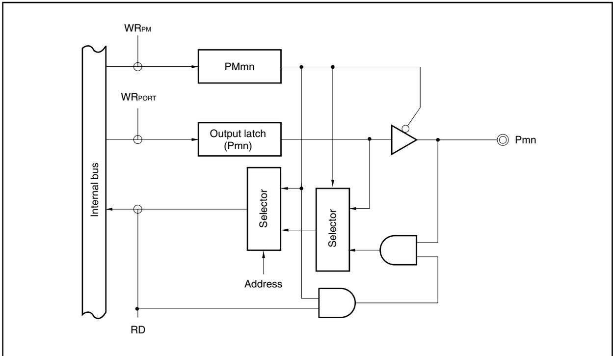
Figure 4-5. Block Diagram of Type C-1
