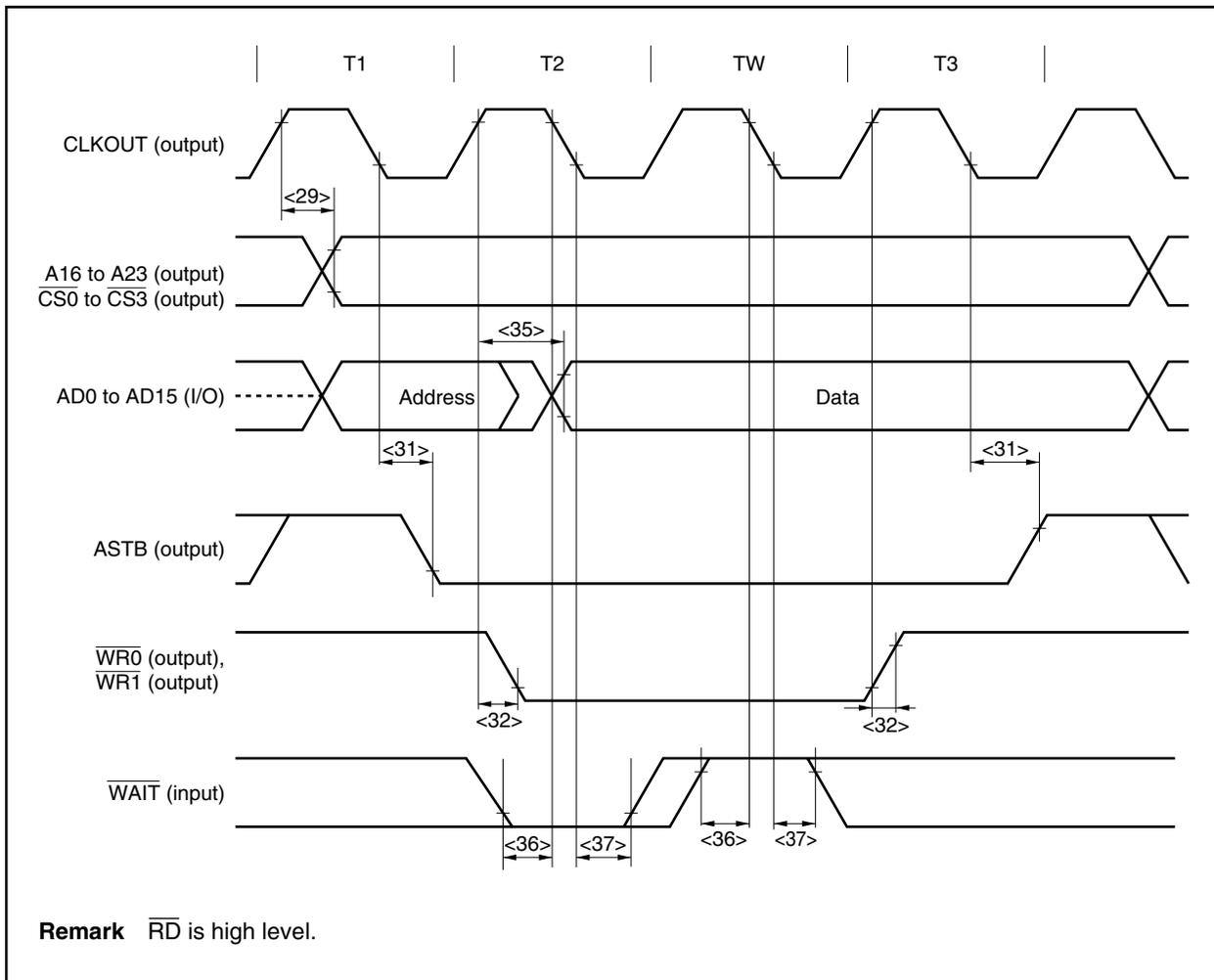
**(2) In separate bus mode****(a) Read cycle (CLKOUT asynchronous): In separate bus mode**
