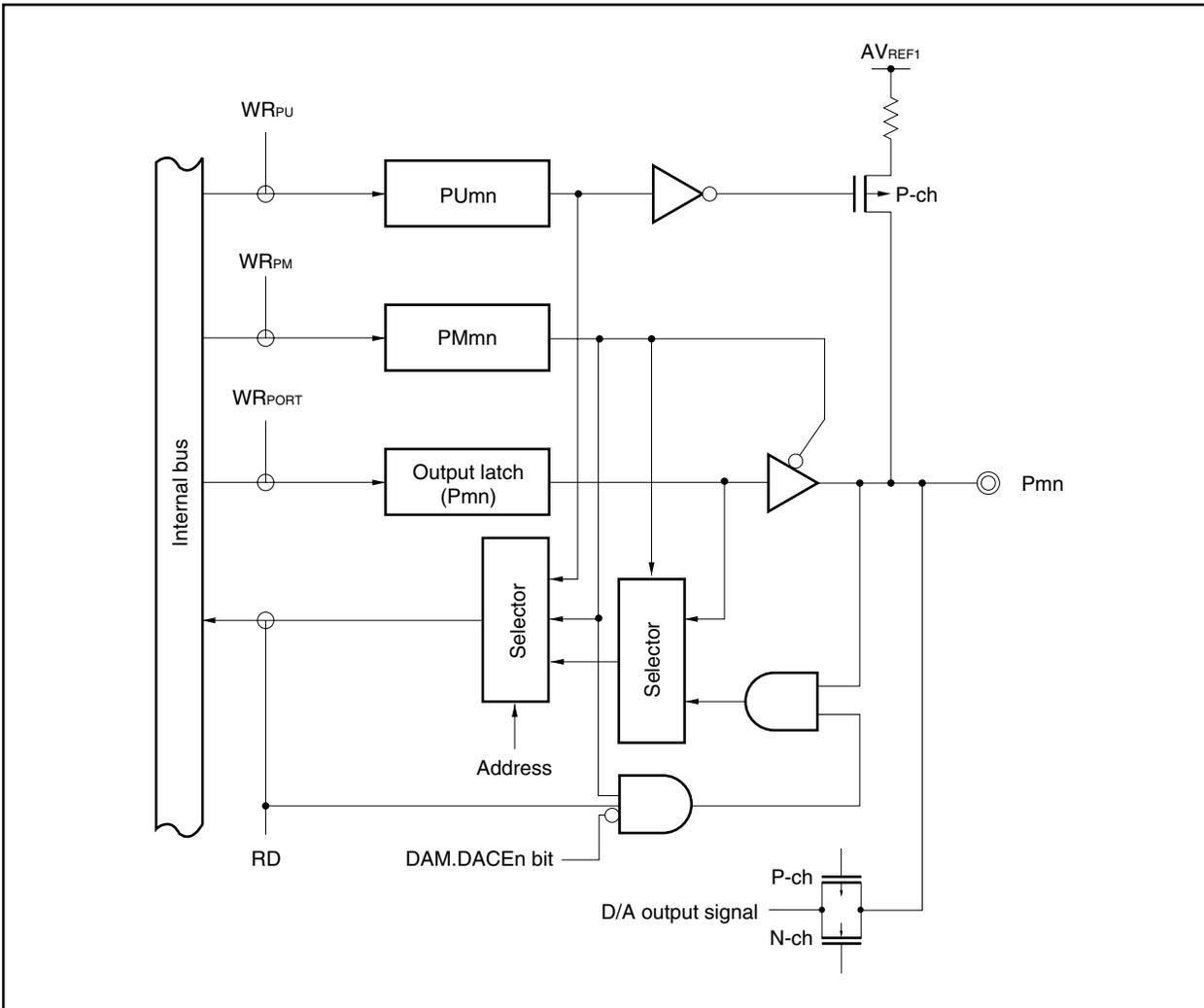
Figure 4-4. Block Diagram of Type B-1
