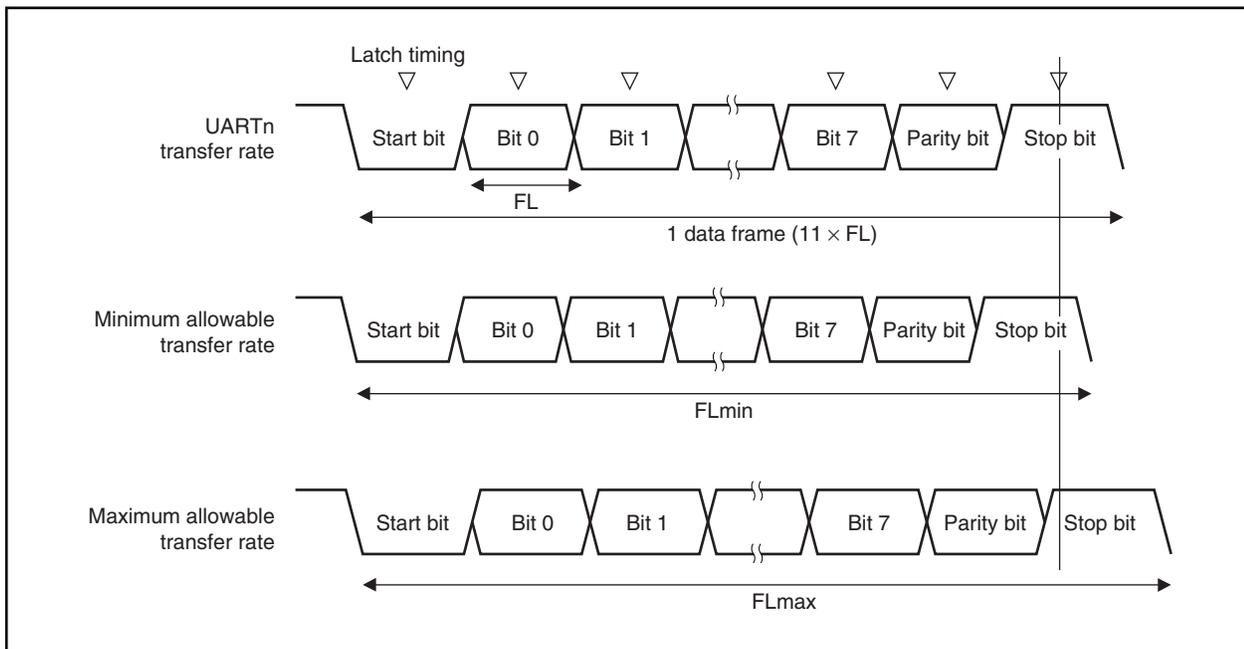
As shown in Figure 16-14, after the start bit is detected, the receive data latch timing is determined according to the counter that was set by the BRGCn register. If all data up to the final data (stop bit) is in time for this latch timing, the data can be received normally.
