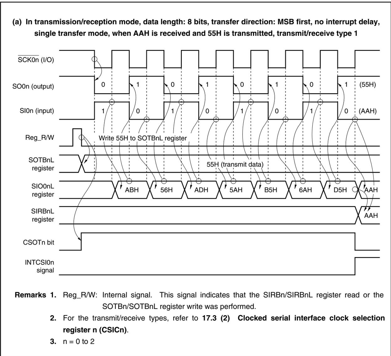
Figure 17-3. Timing Chart in Single Transfer Mode (2/2)
