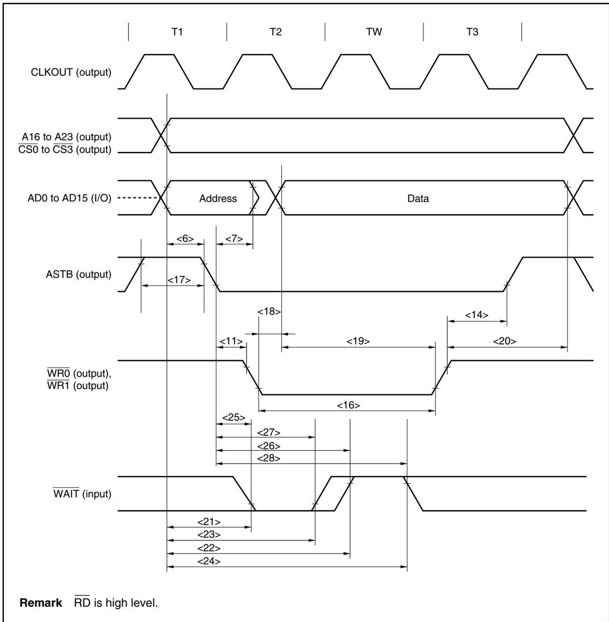
**(b) Read/write cycle (CLKOUT synchronous): In multiplex bus mode**
