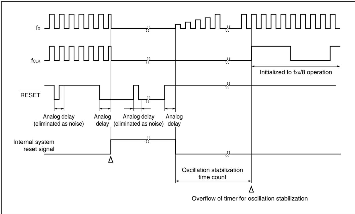
Figure 23-3. Operation on Power Application
