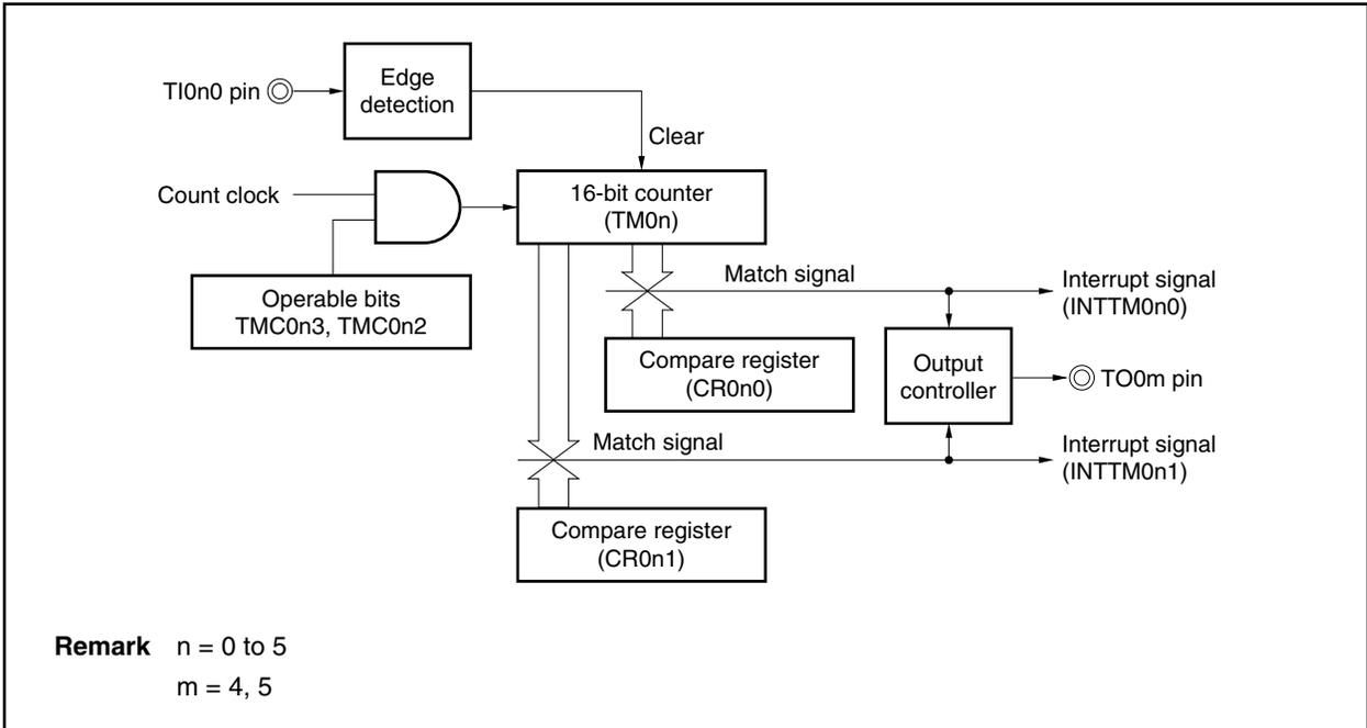
**Figure 8-14. Timing Example of Clear & Start Mode Entered by TI0n0 Pin Valid Edge Input**
