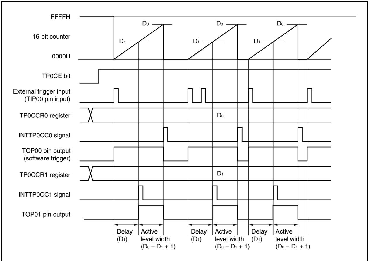
When the TPOCE bit is set to 1, 16-bit timer/event counter P waits for a trigger. When the trigger is generated, the 16-bit counter is cleared from FFFFH to 0000H, starts counting, and outputs a one-shot pulse from the TOP01 pin. After the one-shot pulse is output, the 16-bit counter is set to FFFFH, stops counting, and waits for a trigger. If a trigger is generated again while the one-shot pulse is being output, it is ignored.
