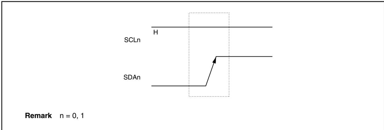
A stop condition is generated when the IICC<sub>n</sub>.SPT<sub>n</sub> bit is set to 1. When the stop condition is detected, the IIC<sub>n</sub>.SPD<sub>n</sub> bit is set to 1 and the interrupt request signal (INTIIC<sub>n</sub>) is generated when the IICC<sub>n</sub>.SPIE<sub>n</sub> bit is set to 1.
