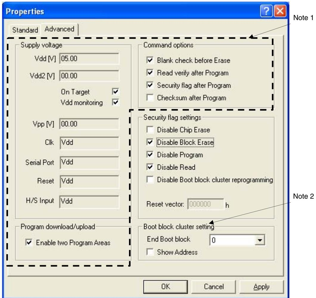
**Notes 1.** Set “Supply voltage”, “Program download/upload”, and “Command potions” in broken lines in accordance with the use conditions.
