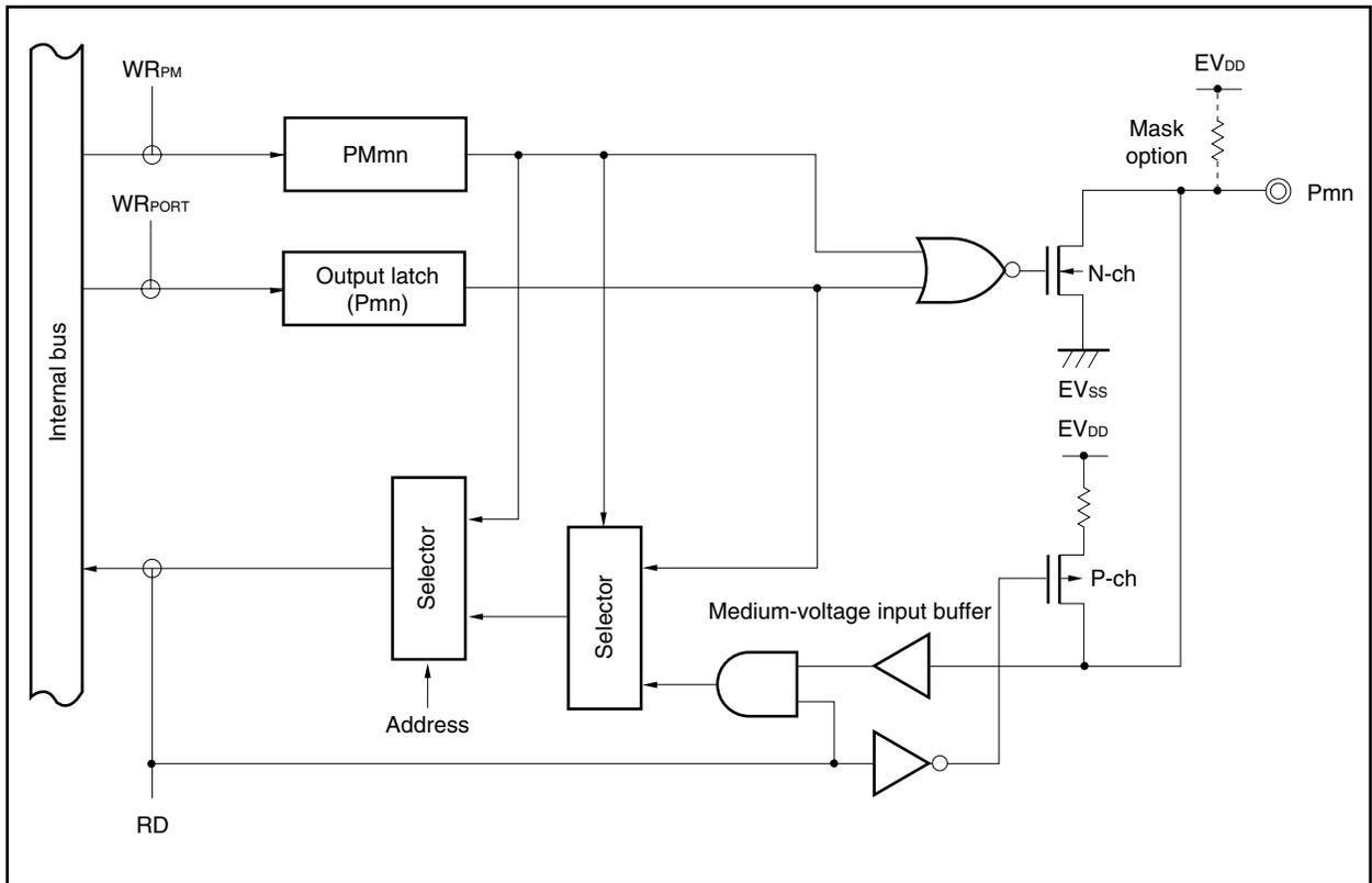
Figure 4-31. Block Diagram of Type K
