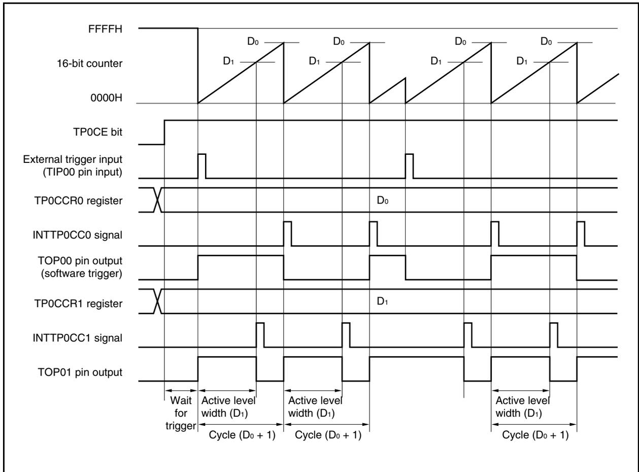
16-bit timer/event counter P waits for a trigger when the TPOCE bit is set to 1. When the trigger is generated, the 16-bit counter is cleared from FFFFH to 0000H, starts counting at the same time, and outputs a PWM waveform from the TOP01 pin. If the trigger is generated again while the counter is operating, the counter is cleared to 0000H and restarted. (The output of the TOP00 pin is inverted. The TOP01 pin outputs a high level regardless of the status (high/low) when a trigger occurs.)
