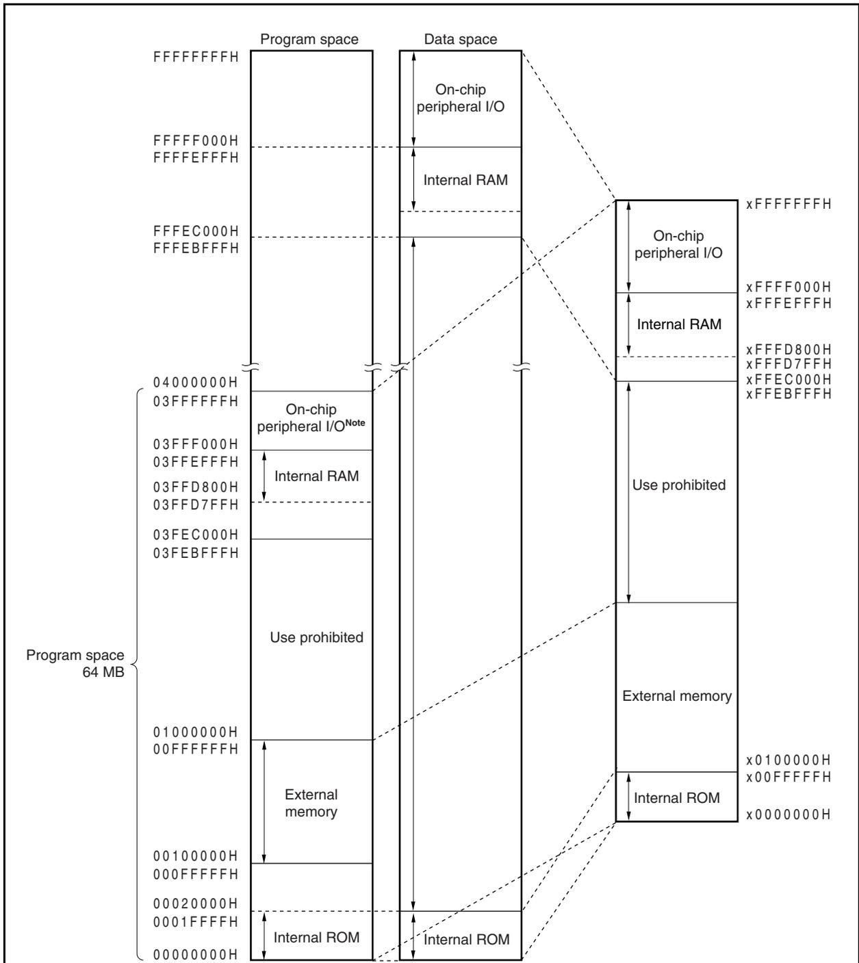
**Note** Access to this area is prohibited. To access the on-chip peripheral I/O in this area, specify addresses FFFF000H to FFFFFFFH.
