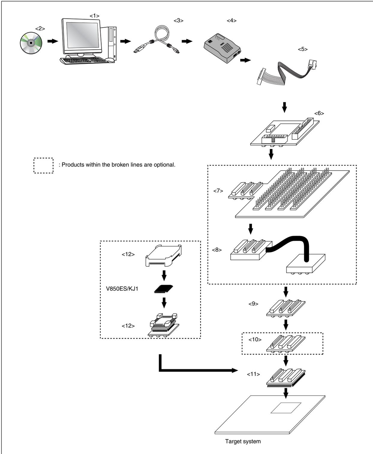
Figure A-5. Example of System Configuration Using QB-V850ESKX1-DA (Not Using Optional Products)
