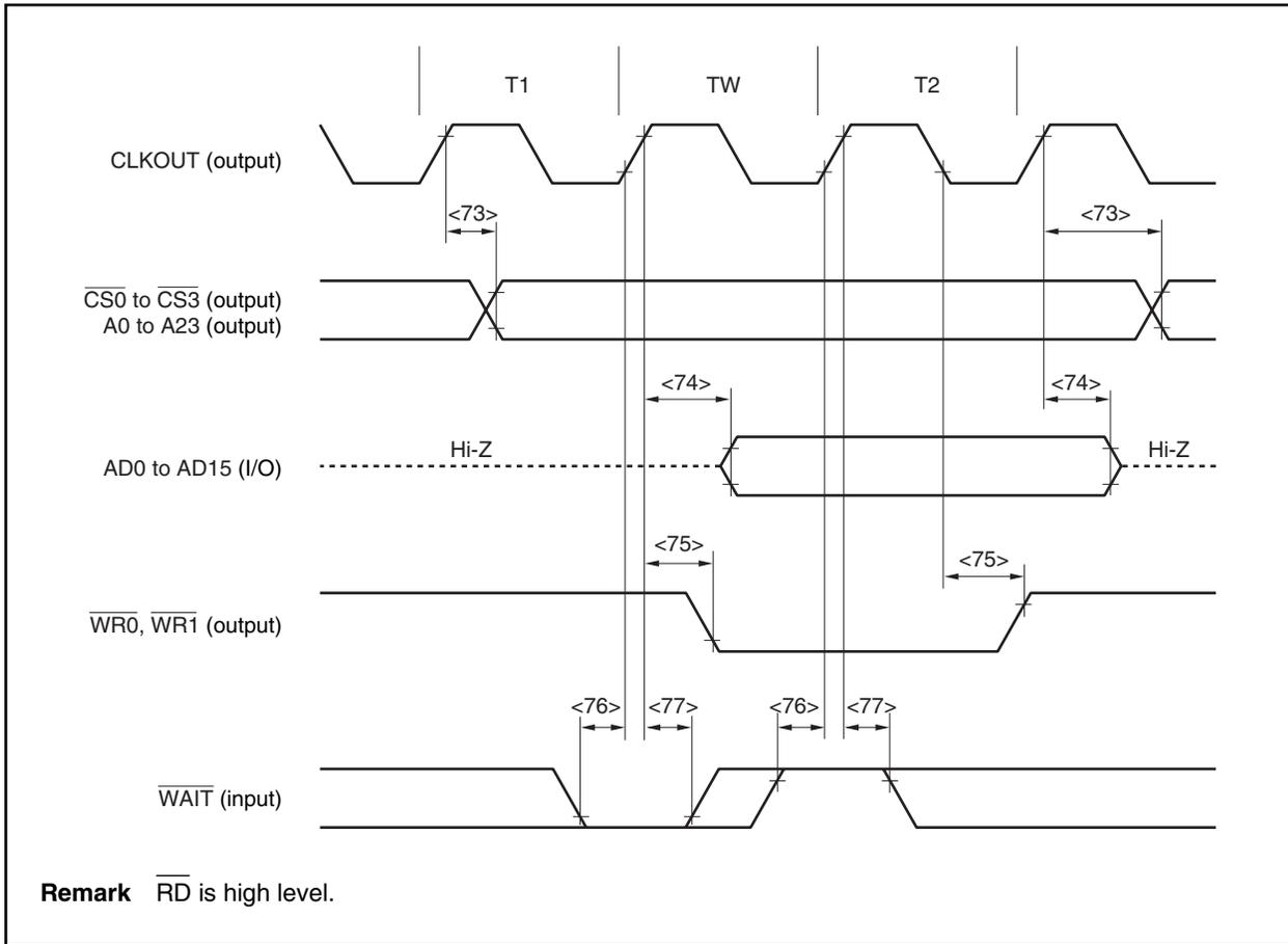
**(3) Bus hold****(a) CLKOUT asynchronous**
