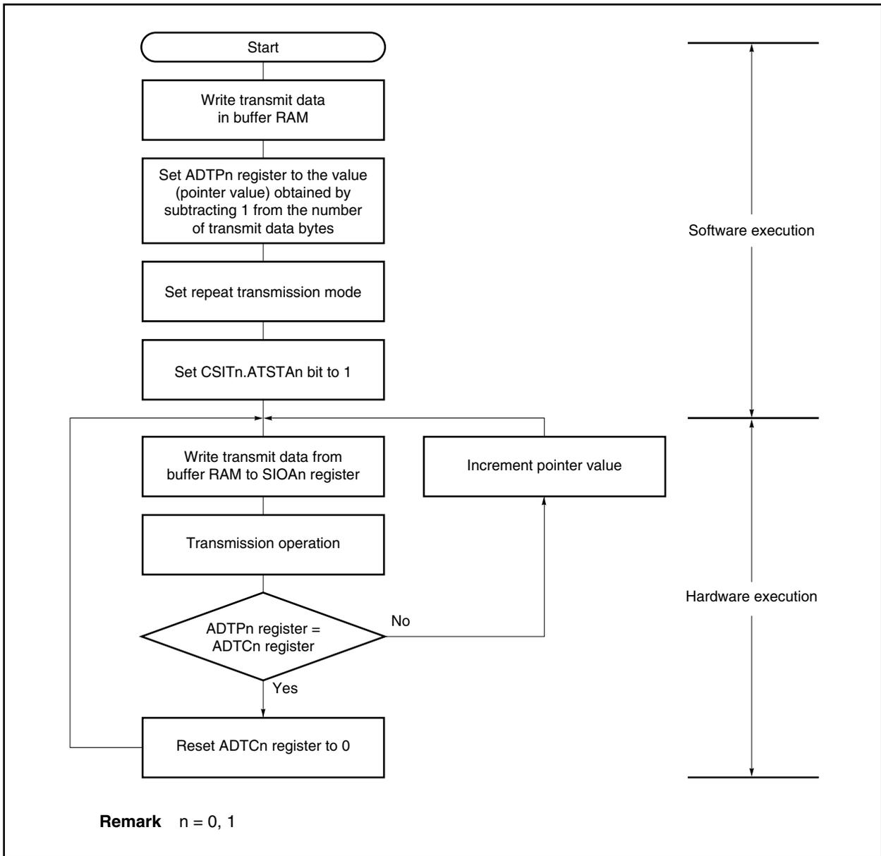
In 6-byte transmission (CSIMAn.ATMn bit = 1, CSIMAn.RXEAn bit = 0, CSIMAn.TXEAn bit = 1, CSIMAn.ATEn bit = 1) in repeat transmission mode, buffer RAM operates as follows.
