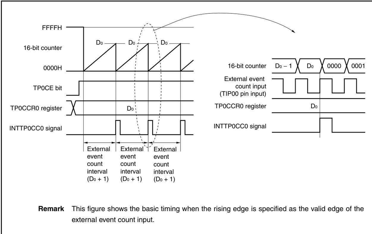
When the TP0CE bit is set to 1, the value of the 16-bit counter is cleared from FFFFH to 0000H. The counter counts each time the valid edge of external event count input is detected. Additionally, the set value of the TP0CCR0 register is transferred to the CCR0 buffer register.
