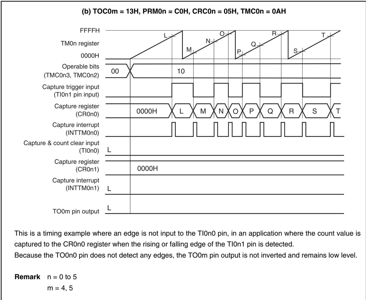
**Figure 8-20. Timing Example of Clear & Start Mode Entered by TIO<sub>n</sub>0 Pin Valid Edge Input (CR0<sub>n</sub> Register: Capture Register, CR0<sub>n</sub>+1 Register: Capture Register) (3/3)**
