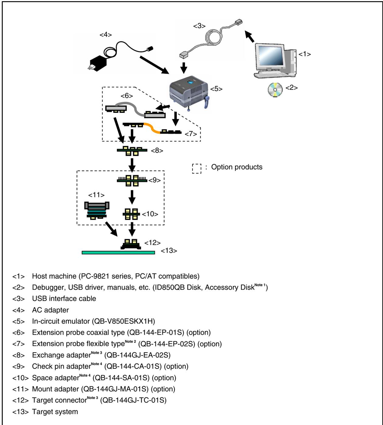
Figure A-2. System Configuration (QB-V850ESKX1H Used) (2/2)
