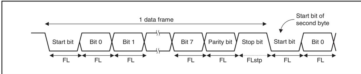
Representing the 1-bit data length by FL, the stop bit length by FLstp, and the base clock frequency by  $f_{\text{uCLK}}$  yields the following equation.
