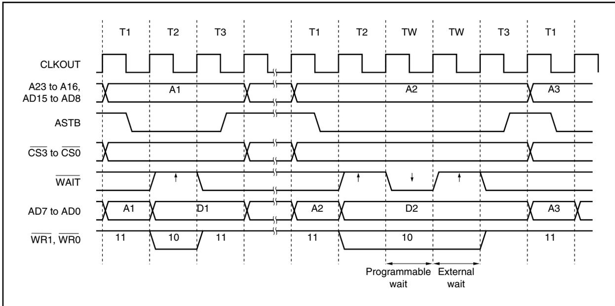
Figure 5-9. Separate Bus Read Timing (Bus Size: 16 Bits, 16-Bit Access)
