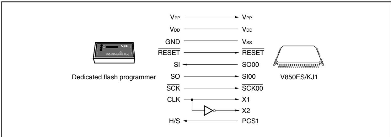
If the PG-FP4 is used as the flash programmer, the PG-FP4 generates the following signals for the V850ES/KJ1. For details, refer to the **PG-FP4 User's Manual (U15260E)**.
