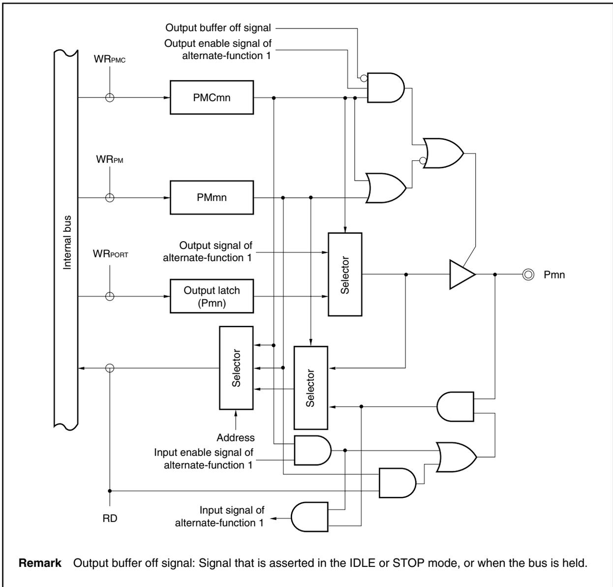
Figure 4-9. Block Diagram of Type D-1-1
