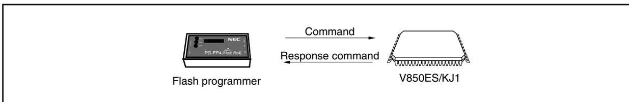
The flash memory control commands of the V850ES/KJ1 are listed in the table below. All these commands are issued from the programmer and the V850ES/KJ1 performs processing corresponding to the respective commands.
